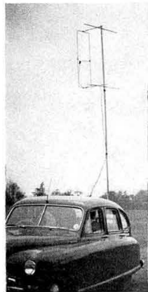
G5ML's single slot for two metres at a height of 16 ft was one of the more ambitious mobile aerial systems seen at the Rally.
